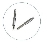
Our Banana plugs are machined from non-magnetic solid bar, then fitted with a spring tension 'lantern' at the tip to provide a reliable, constant contact with the socket of any standard 4mm enrty binding post. As with all of our connectors, they are heavily plated with high purity Silver. Cable connection is via soldering, and a deep solder bucket is machined into the rear of the plug. They are not colour coded, so appropriate heatshrink markers will need to be applied during installation.
