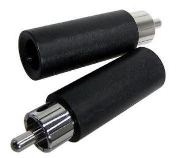
These exquisite plugs can receive cables up to 7.9mm in diameter, their overall diameter is 13mm and their length is 46mm. The outer shell screws onto the main portion. Additionally, a grub screw contact provides superb physical contact onto the main cable.
