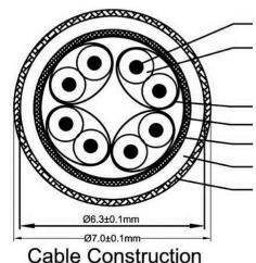
Main conductor: 24 AWG Silver plated  $\alpha$  (Alpha) OCC conductor Insulation: Special Foamed PE OD.: 1.35 $\pm$ 0.05mm, 4 Twisted Pairs Blue/White; Orange/White; Green/White; Brown/White
