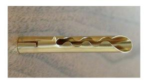
Our **banana plugs** are manufactured using a special byrillium copper sheet and subsequently gold plated. The byrillium gives the copper the necessary spring tension that is needed in order to ensure a high contact pressure when in contact with a socket and therefore guaranteeing security. The acoustic advantages of copper remain largely unaffected.
