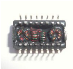
The actual transformers are tiny toriod's, inside an SMD package.
