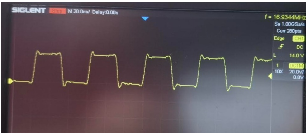
The 16.9344 MHz clock signal, set to 3.3Vpp setting.
