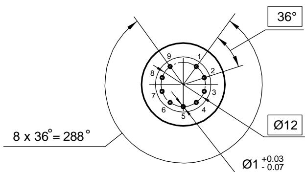
Electrode -to - lead connection diagram
