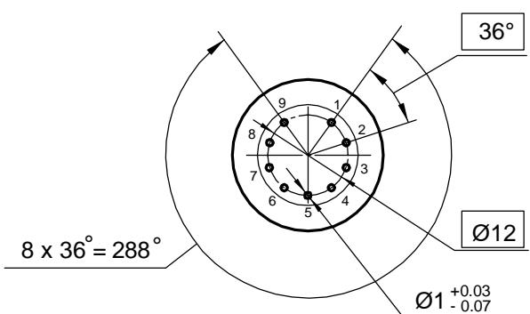
Electrode -to - lead connection diagram
